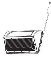
2. Step 2: Separate the male and female connectors, and then remove the reflector from the back plate.
