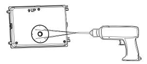
4. **Step 4:** Run the main power wire from the water-proof J-box through the middle hole, then lock the back plate to the wall using appropriate screws.
