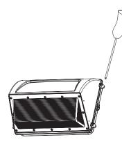
2. Step 2: Separate the male and female connectors, and then remove the reflector from the back plate.
