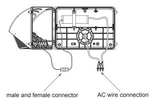
6. **Step 6:** Use a suitable screwdriver to connect the reflector to the back plate by tightening screws. The installation is finished.
