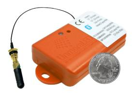
The ULPLUS is a Bluetooth NLC Wireless Receiver and Fixture Controller for fixtures that don't require motion sensors.
