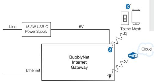
For best results, Gateways need to be installed within 30 feet of the closest device within the Mesh network. Signal strength significantly decreases in presence of metal barriers such as when devices are enclosed in metal boxes.
