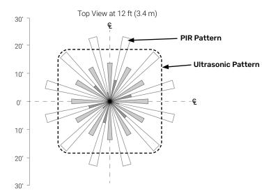
Note: The application/absolute range of the sensor is subject to variation because of different types of clothing, backgrounds, and ambient temperature. Therefore, ensure the lens is properly oriented along routes with expected traffic and conduct testing along those routes.
