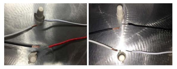
Step 5: The LED Driver comes standard with 0-10 Volt Dimming. The Red, Purple, and Grey wires on the output side of the driver are for dimming functions. If the dimming functions will not be used, leave the quick disconnect on the 3 wires.
