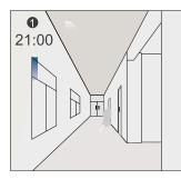
The fixture turns **On** at 100% when motion is detected.
