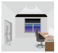
After hold time, the fixture **Dims** to stand-by level if natural light stays below daylight threshold.
