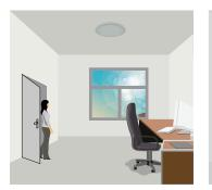
With sufficient natural light, even when motion is detected, the fixture remains **Off**.
