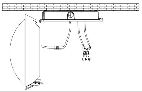
6. **Step 6:** Fixate the fixture housing to the back plate firmly with buckle. The installation is finished.
