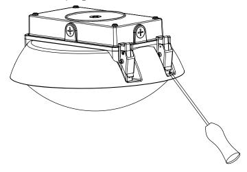
2. **Step 2:** Disconnect the male and female connectors, and then remove the fixture housing from the back plate.
