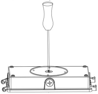
4. **Step 4:** Lock the back plate to the 1/2" threaded conduit pipe.
