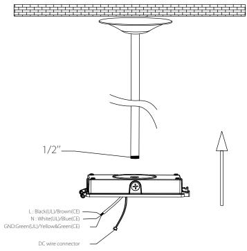
5. **Step 5:** Lock the fixture housing. Re-connect the DC male and female connectors. AC wire connections with wire nut.
