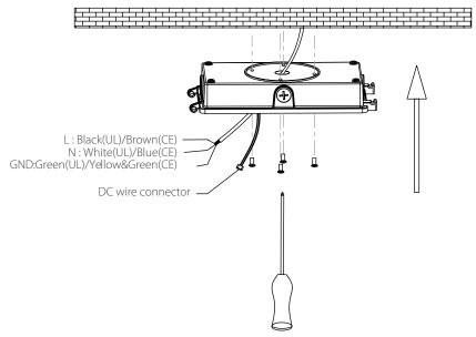
5. **Step 5:** Lock the fixture housing. Re-connect the DC male and female connectors. AC wire connections with wire nut.
