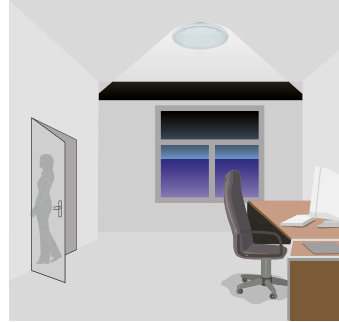
After hold time, the fixture Dims to stand-by level if natural light stays below daylight threshold.
