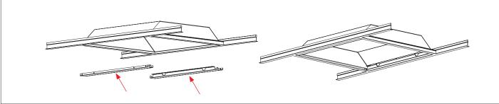
4. Hook the troffer retrofit kit body to the existing frame through the clasps in body to the sidemounting bracket.
