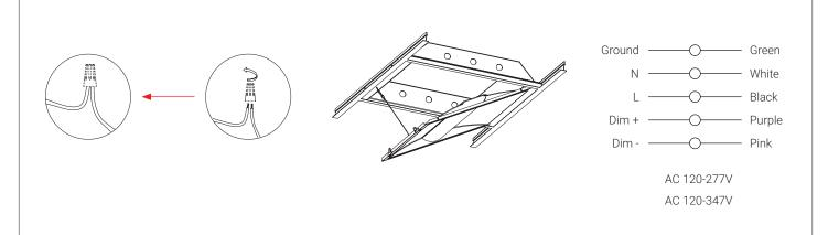
8. Rotate retrofit kit into body toward the side mounting brackets.
