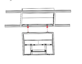
5. Make sure the doorkit is clamped tightly to the side-mounting bracket.
