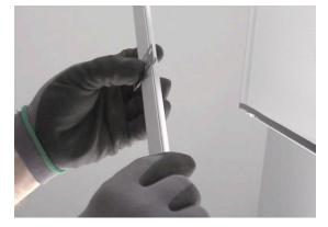
**Step 3:** While light bars are magnetically attached only, align light bar screw holes to desired placement. Then secure with provided self-tapping screws.
