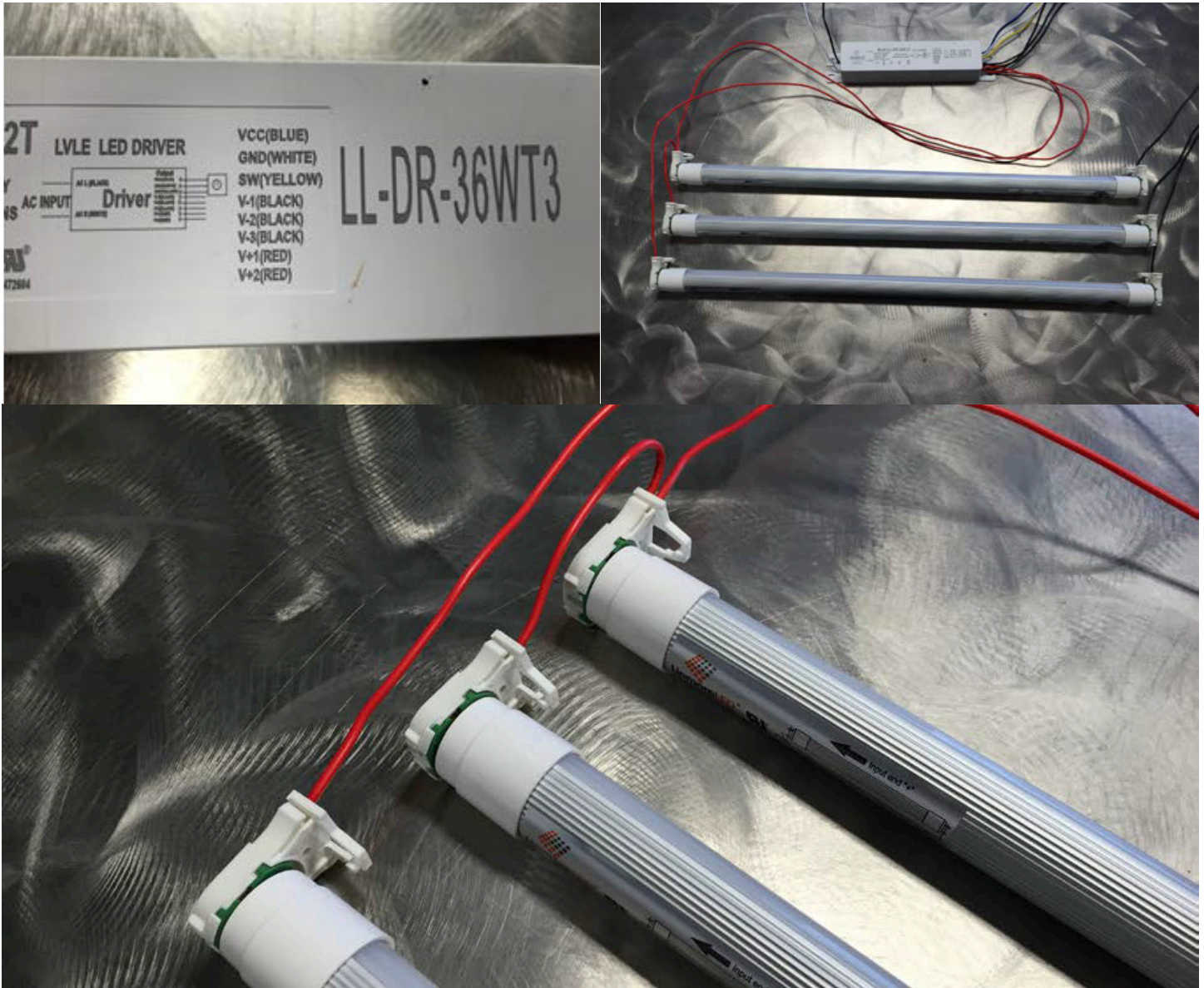
3 Tubes: 5 Driver Output Leads: 2 Red/Positive/+ and 3 Black/Negative/-
