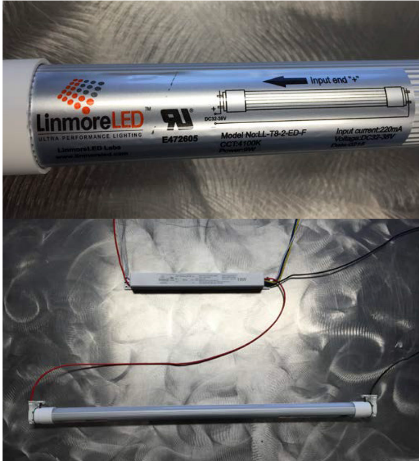
1 Tube: 2 Driver Output Leads: 1 Red/Positive/+ and 1 Black/Negative/-
