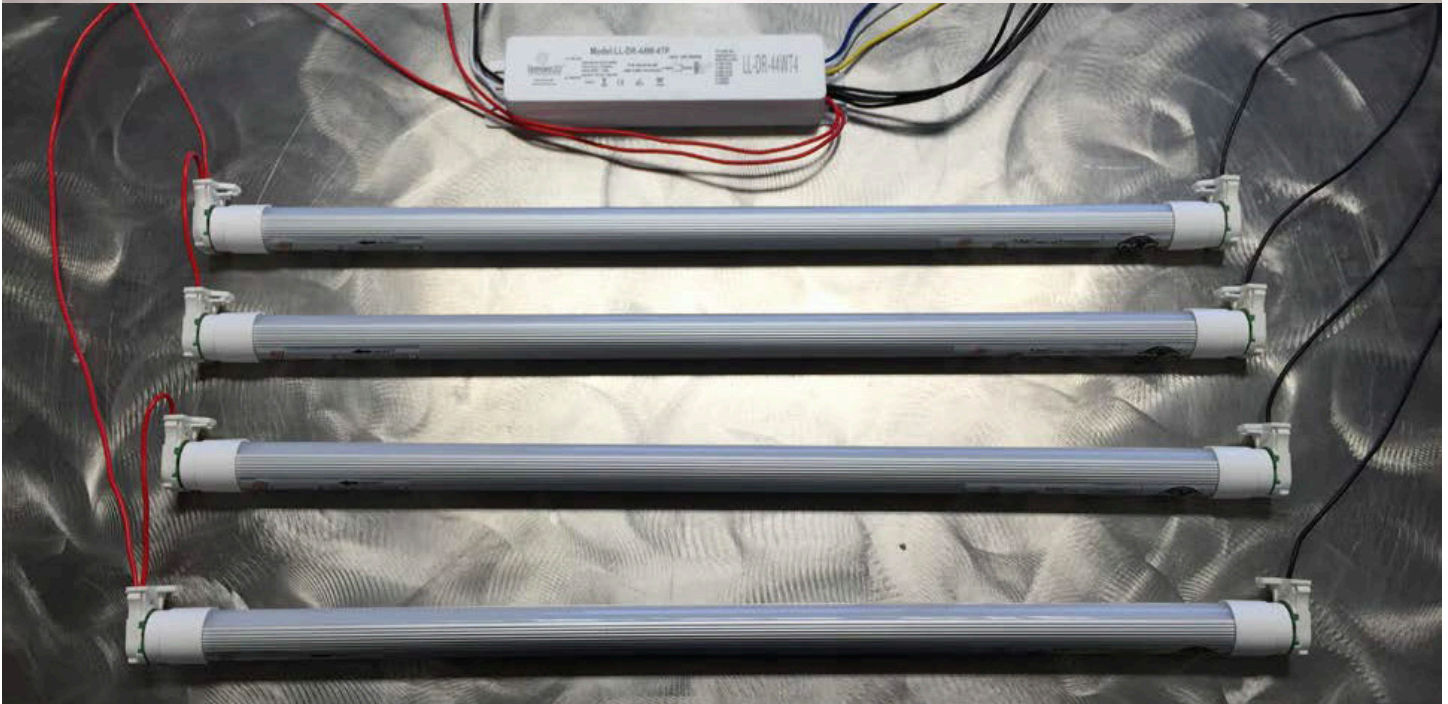
4 Tubes: 6 Driver Output Leads: 2 Red/Positive/+ and 4 Black/Negative/-
