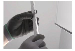
3. **Step 3:** While light bars are magnetically attached only, align light bar screw holes to desired placement. Then secure with provided self-tapping screws.
